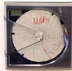
Close-up of recorder showing 7 day temperature and humidity digital display
